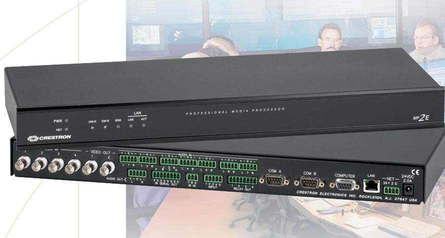
The MP2E is a low-cost 2-Series Ethernet control system and audio/video switcher that provides total control of a room's multi-media resources, including CD players, DVD players, projectors, screens, even lighting. With a unique combination of high-performance Ethernet control and switching at an affordable price, the MP2E is the ideal AV control solution for colleges, corporate campuses, and other multi-room facilities.
